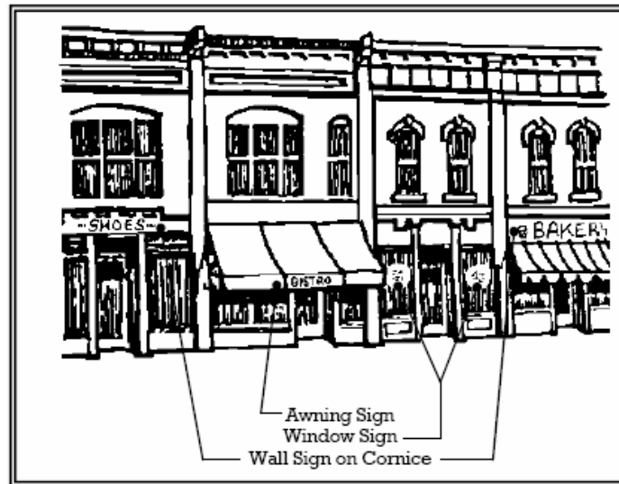
Figure 12 - Historical Wall and Awning Signage Applications
