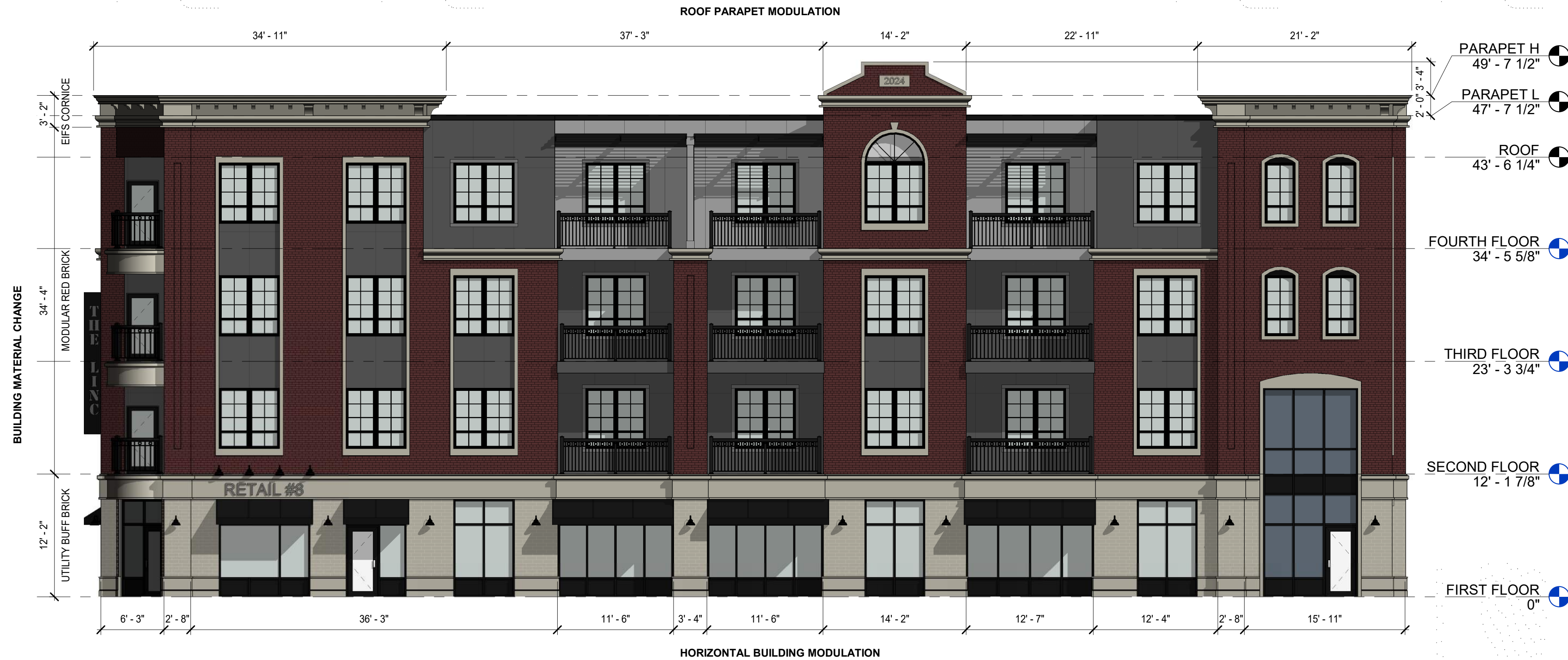
2 BUILDING B - EAST ELEVATION - MORGAN BLVD 1/8" = 1'-0"
