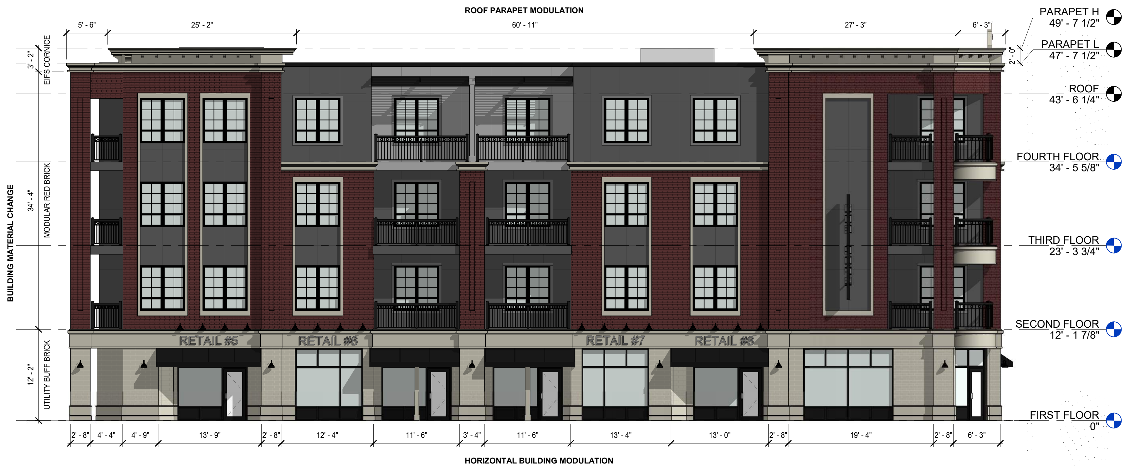
1 BUILDING B - SOUTH ELEVATION - LINCOLNWAY 1/8" = 1'-0"
