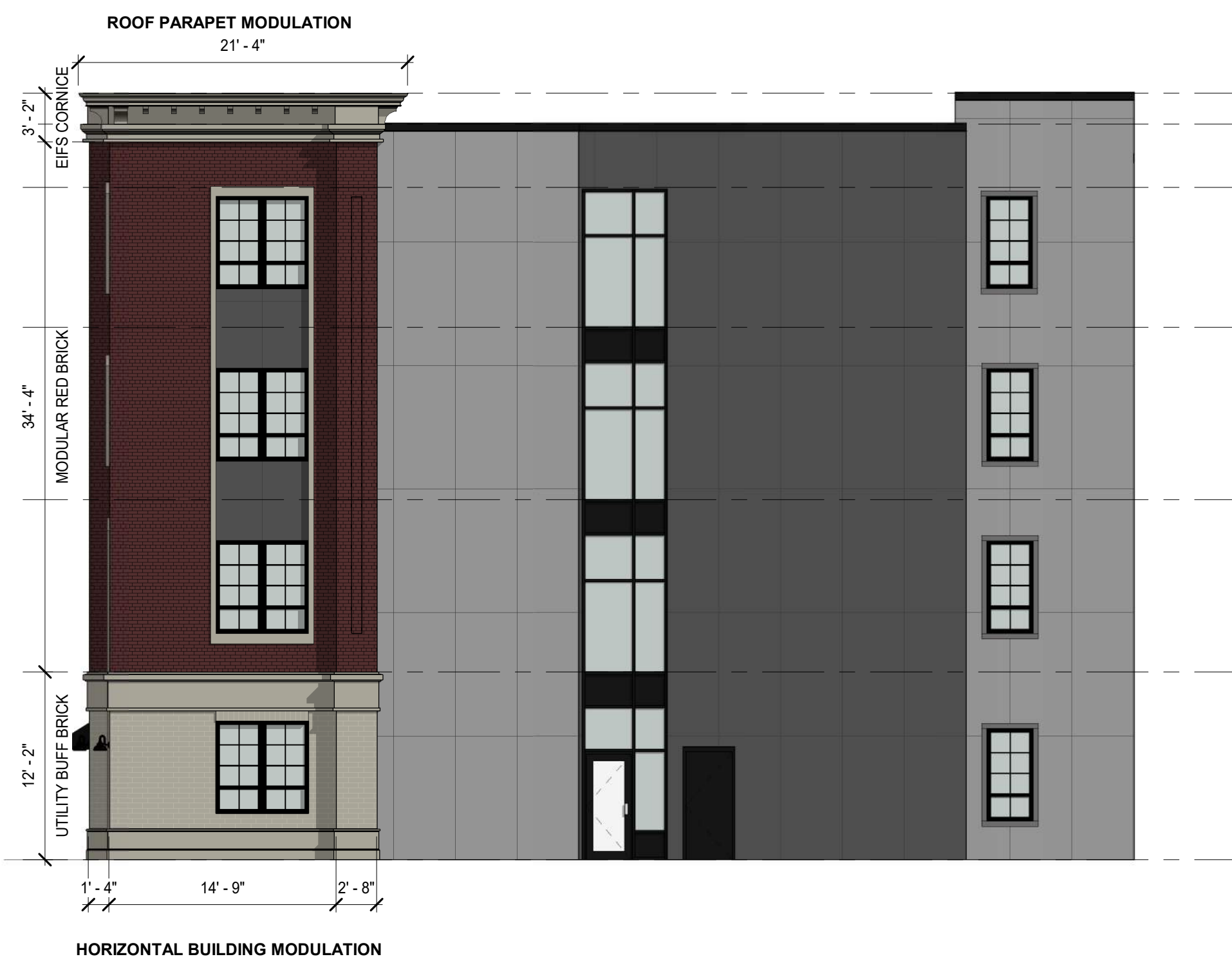
3 BUILDING B - NORTH ELEVATION - ALLEYWAY 1/8" = 1'-0"
