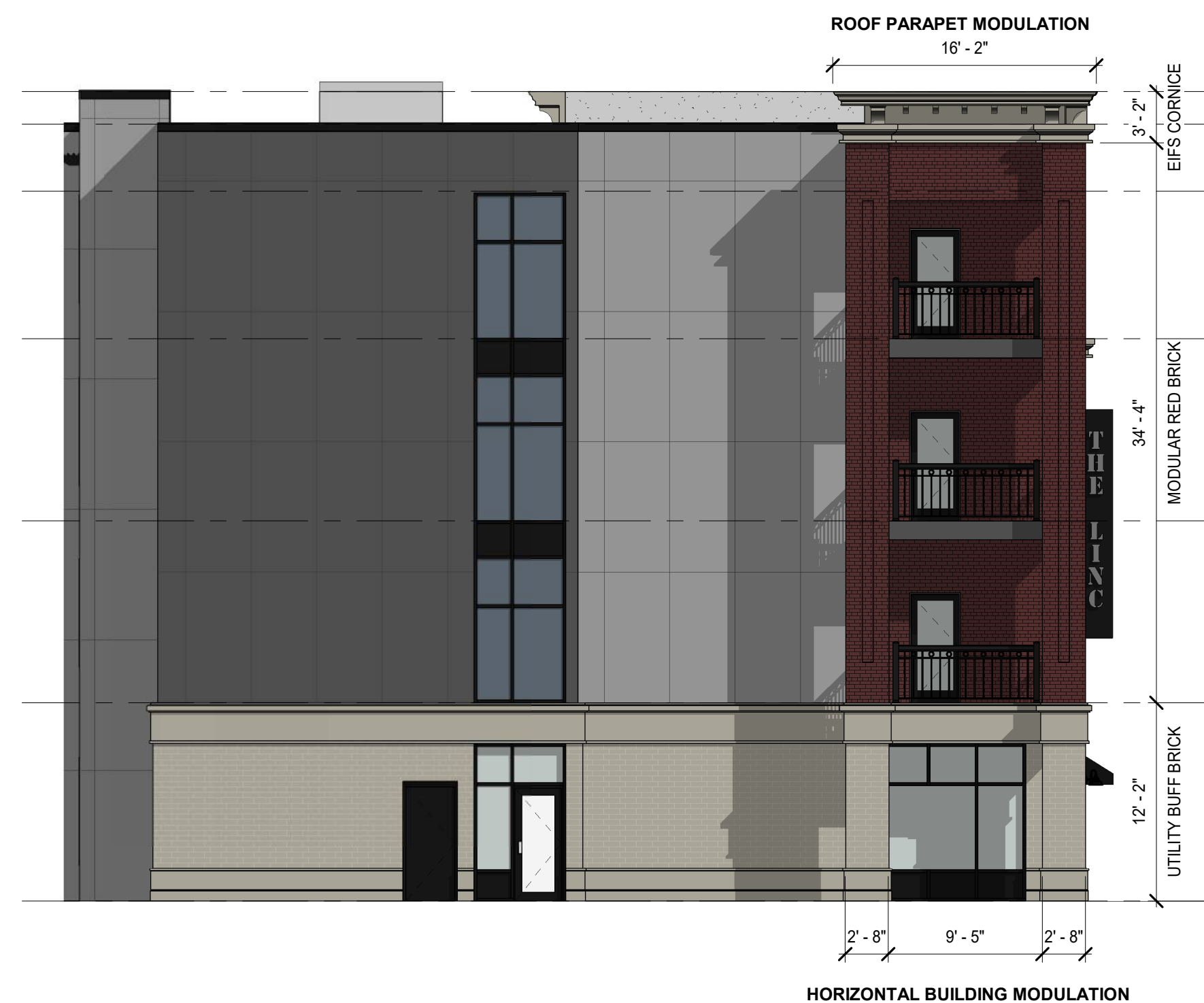
4 BUILDING B - WEST ELEVATION - ALLEYWAY 1/8" = 1'-0"
