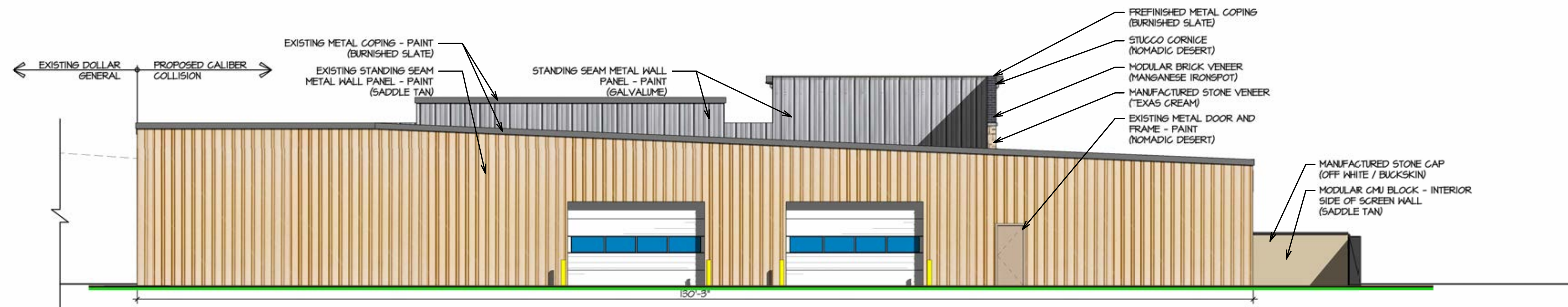
2 PRELIMINARY WEST ELEVATION 1/8" = 1'-0" 0 4' 8' 16' SCALE: 1/8" = 1'-0"
